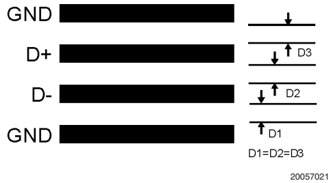
FIGURE 10. Ideal Diode Trace Layout
