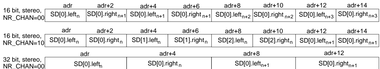
Figure 2: Examples of Audio Out Memory DMA Formats
