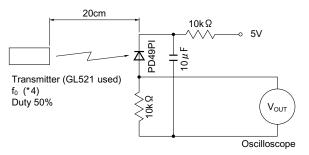
In the above figure, the transmitter should be set so that the output V<sub>OUT (P-P)</sub> can be 40mV. However, the PD49PI to be used here should be of the short-circuit current Isc=2.6  $\mu$  A at Ev =100 Ix. (E<sub>v</sub> is an illuminance by CIE standard light source A (tungsten lamp).)
