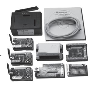
networks. It features a 250 kbps high data rate and utilizes a direct sequence spread spectrum radio that is generally resistant to RF interference and provides enhanced data security. Plug and play software includes pre-installed mesh networking firmware and an intuitive sensor network user interface.
