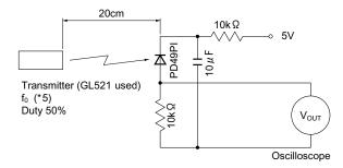
In the above figure, the transmitter should be set so that the output VouT (P-P) can be 40mV. However, the PD49PI to be used here should be of the short-circuit current Isc=2.6  $\mu$  A at Ev =100 Ix. (E<sub>V</sub> is an illuminance by CIE standard light source A (tungsten lamp).)
