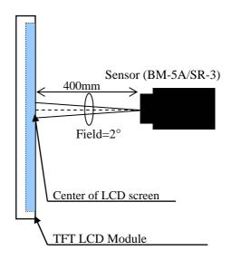
Fig.9-2 Measuring setup for
