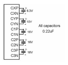
Note 3) Stabilization and charge sharing Capacitors
