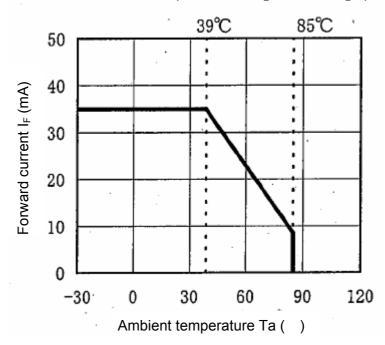
Ambient temperature of LED and the maximum input
