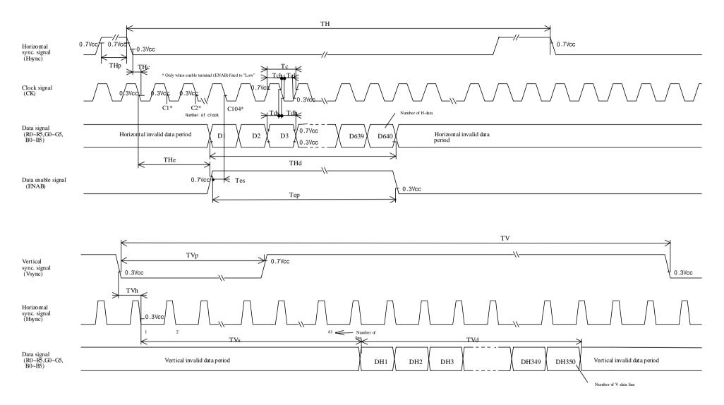
Fig.2-3 Input signal waveforms (350 line mode)
