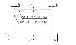
1. UNSPECIFIED TOLERANCE TO BE  $\pm 0.5$ 2. PLEASE DESIGN USER' S CABINET BOSSES WITH 6mm TO 8mm IN DIAMETER.
