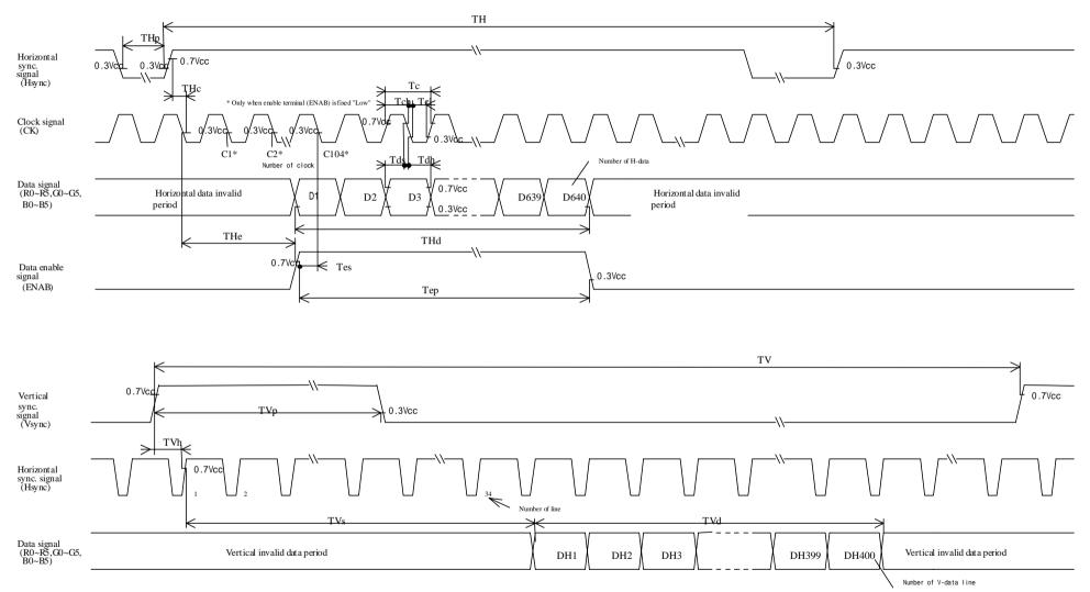
Fig.2-2 Input signal waveforms (400 line mode)
