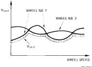
$V_{\text{OUT}}$  is proportional to the lower of the two input wheel speeds.
