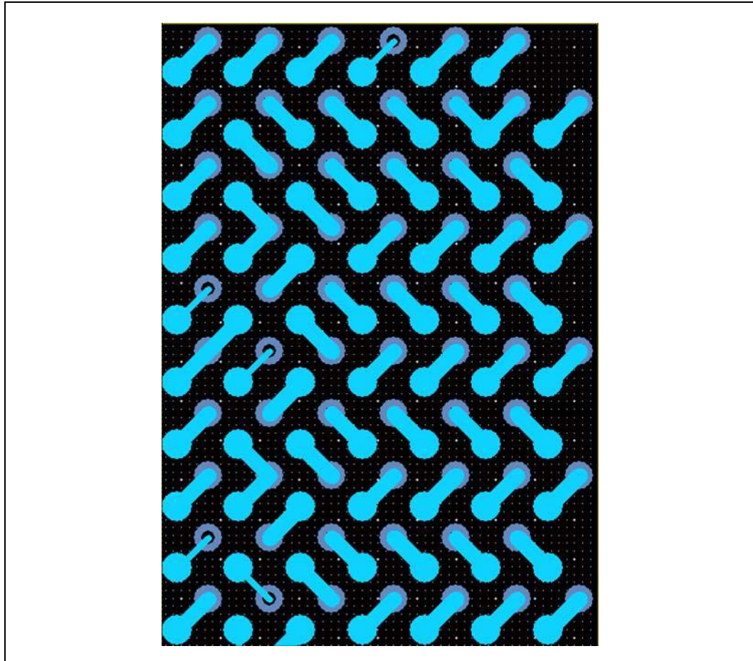
Figure 10. Rambus* Controller Footprint and Via Placement Showing Exploded View of Checkerboard Detail
