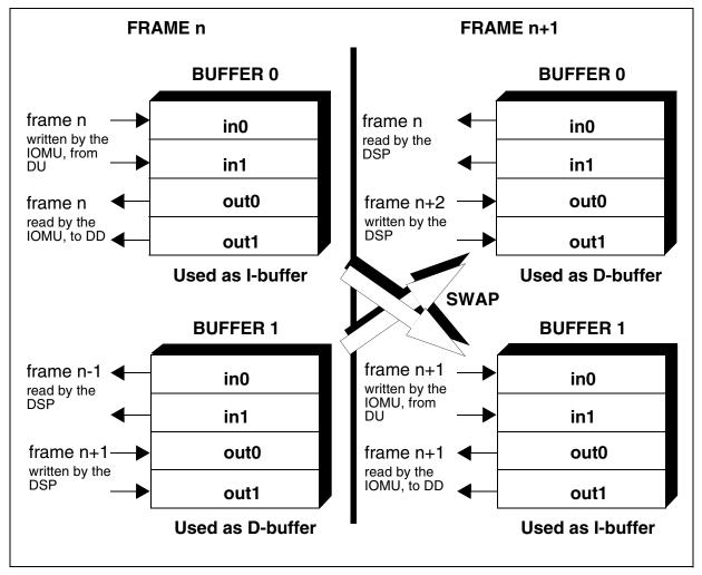
Figure 35 The Circular-Buffer During two Consecutive Frames
