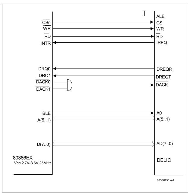
Figure 92 DELIC Connection to Intel 80386EX (Demuxed Configuration)
