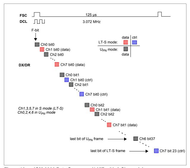
Figure 12 IOM-2000 Data Sequence (1 VIP with 8 Channels)
