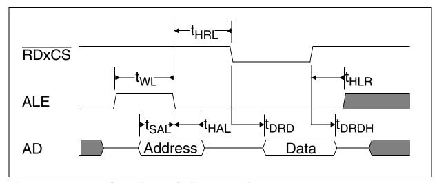
Figure 68 Read Cycle in Intel/Infineon Multiplexed Mode
