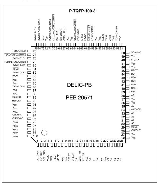
Figure 10 Pin Configuration DELIC-PB
