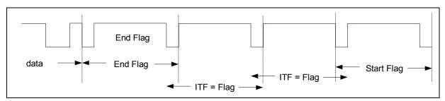
Figure 50 Interframe Time Fill with shared Zero
