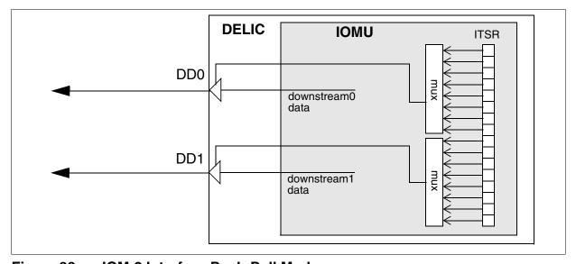
Figure 38 IOM-2 Interface Push-Pull Mode
