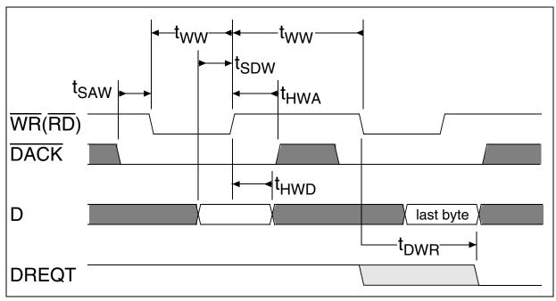
Figure 61 DMA Write-Transaction Timing in Intel/Infineon Mode
