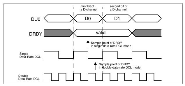
Figure 40 DRDY Sampling Timing
