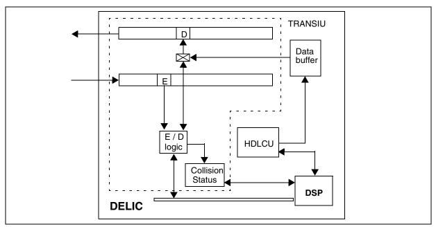
Figure 31 Collision Detection in the LT-T Mode
