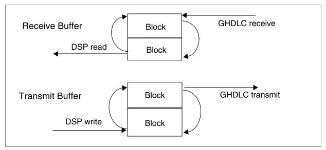
Figure 49 GHDLC Receive and Transmit Buffer Structure
