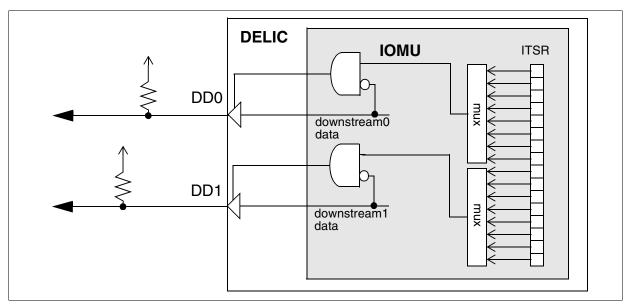
Figure 37 IOM-2 Interface Open-Drain Mode
