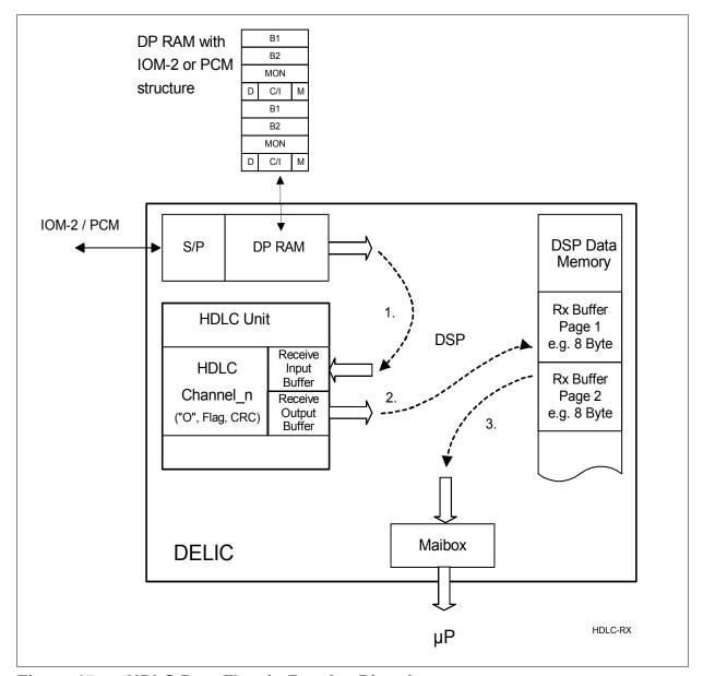
Figure 45 HDLC Data Flow in Receive Direction
