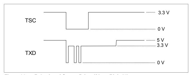
Figure 96 Behavior of Output Driver if Last Bit is '1'
