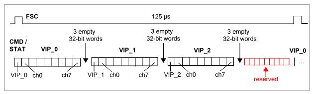
Figure 15 IOM-2000 Command/Status Sequence (3 VIPs with 24 Channels)
