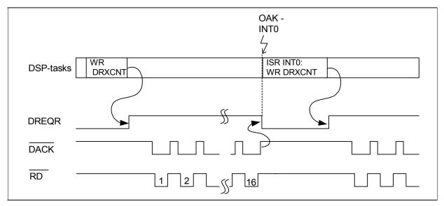
Figure 56 Timing in two-cycle DMA Mode for Receive Direction and Infineon/
