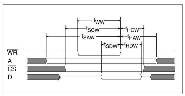
Figure 65 Write Cycle Intel/Infineon Demultiplexed Mode
