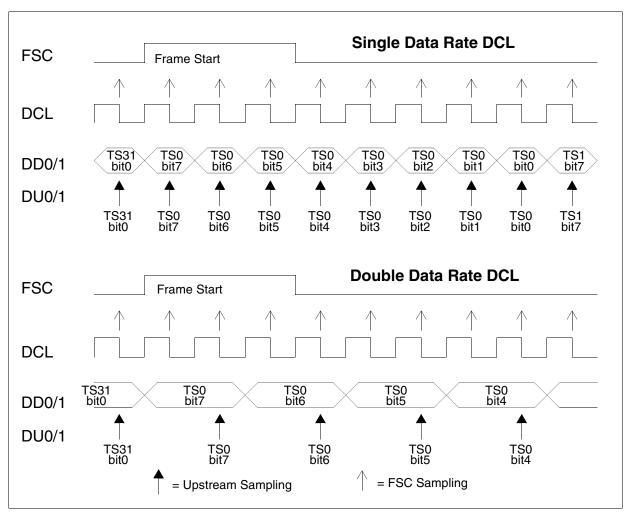
Figure 36 IOM-2 Interface Timing in Single/Double Clock Mode
