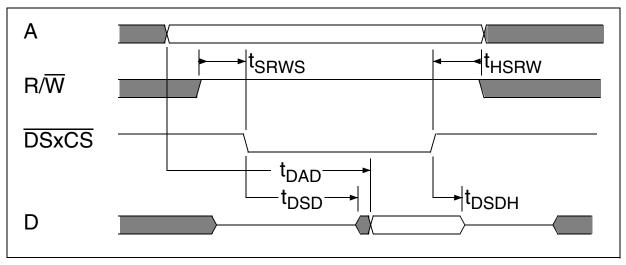
Figure 64 Read Cycle Motorola Mode
