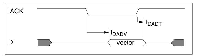
Figure 69 Interrupt Acknowledge Cycle Timing in Motorola Mode
