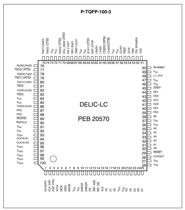
Figure 9 Pin Configuration DELIC-LC
