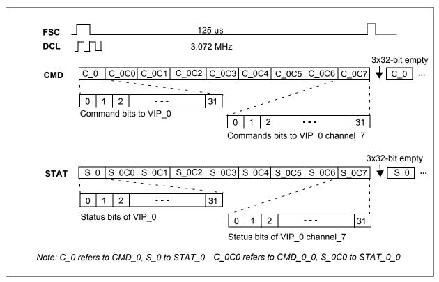
Figure 14 IOM-2000 CMD/STAT Handling (1 VIP with 8 Channels)
