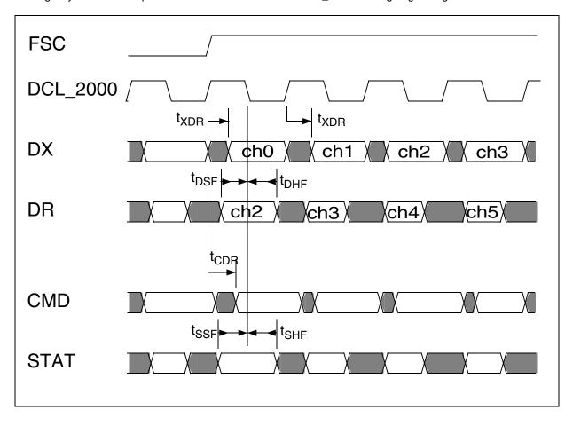
Figure 81 IOM-2000 Interface Timing
