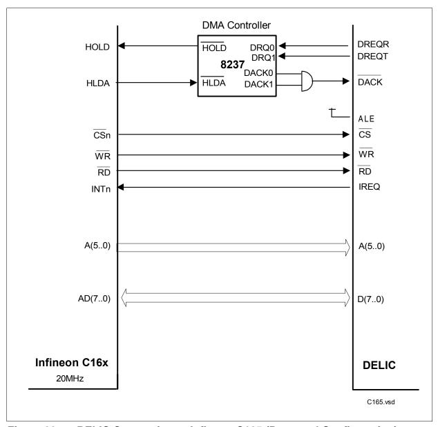
Figure 93 DELIC Connection to Infineon C165 (Demuxed Configuration)
