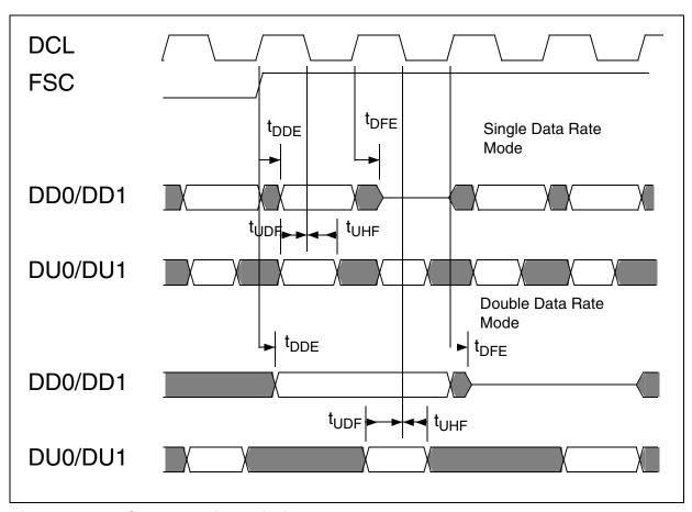
Figure 72 IOM-2 Interface Timing
