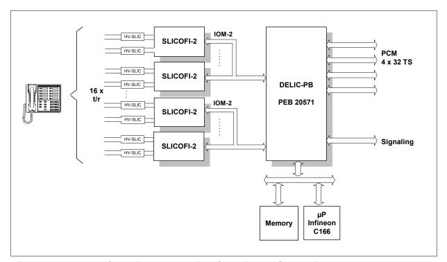
Figure 6 DELIC-PB in Analog Line Card for 16 Subscribers
