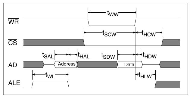
Figure 67 Write Cycle Intel/Infineon Multiplexed Mode
