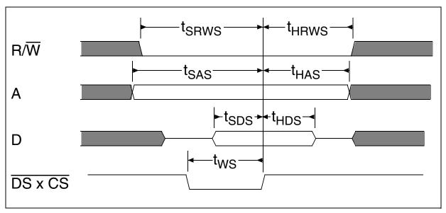
Figure 63 Write Cycle Motorola Mode
