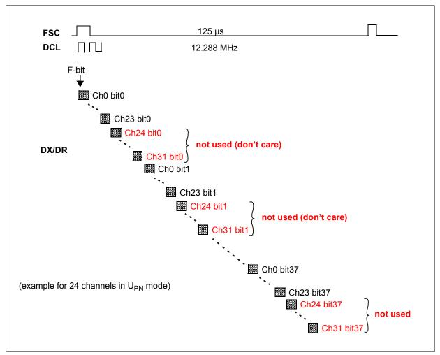
Figure 13 IOM-2000 Data Order (3 VIPs with 24 Channels)
