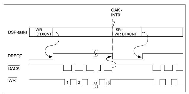
Figure 55 Timing in two-cycle DMA Mode for Transmit Direction and Infineon/
