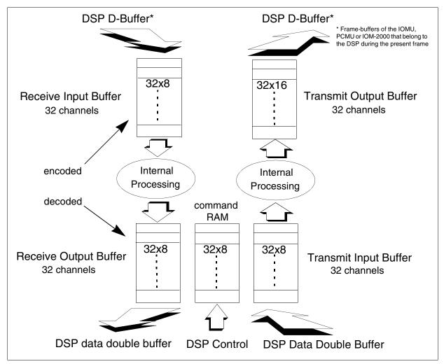
Figure 44 HDLCU General Block Diagram
