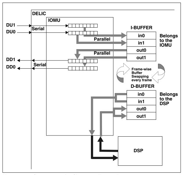
Figure 34 IOMU Frame-Wise Circular-Buffer Architecture
