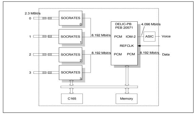
Figure 8 DELIC-PB in 4 Port SDSL Line Card
