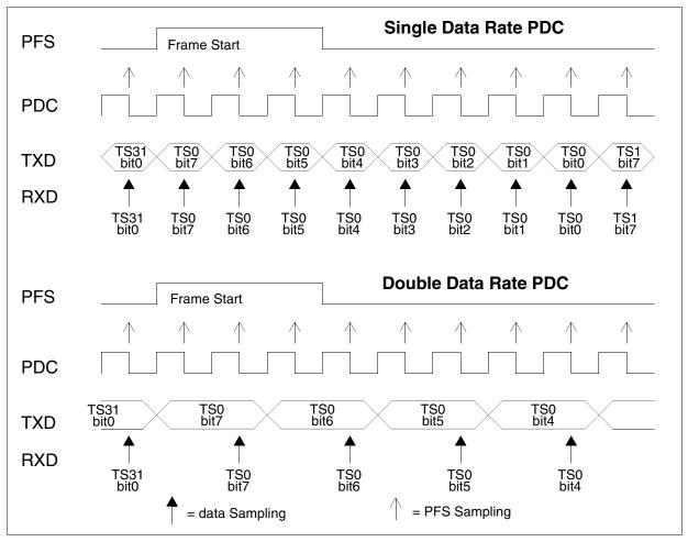
Figure 42 IOM-2 Interface Timing in Single/Double Clock Mode
