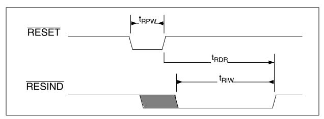
Figure 87 Reset Indication Timing
