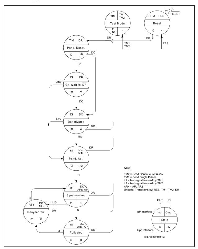
Figure 16 U<sub>PN</sub> State Diagram
