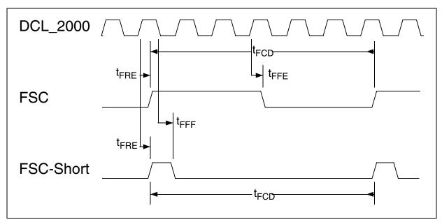
Figure 82 FSC Timing IOM-2000
