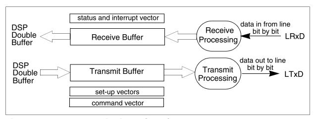
Figure 46 Data Processing in the GHDLC
