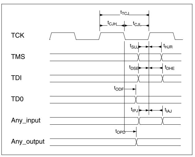
Figure 86 Test-Interface (Boundary Scan) Timing
