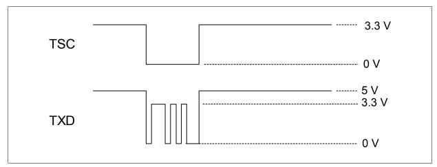
Figure 97 Behavior of Output Driver if Last Bit is '0'
