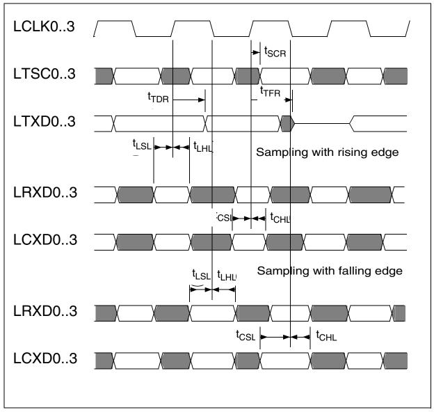
Figure 83 LNC0..3 (Local Network Controller) Interface Timing
