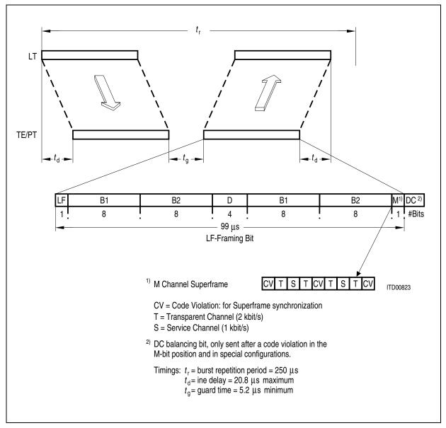
Figure 22 U<sub>PN</sub> Interface Frame Structure
