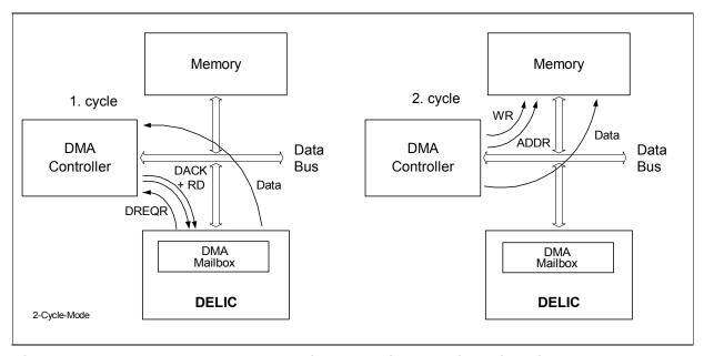
Figure 52 Two-cycle DMA Transfer Mode for Receive Direction
