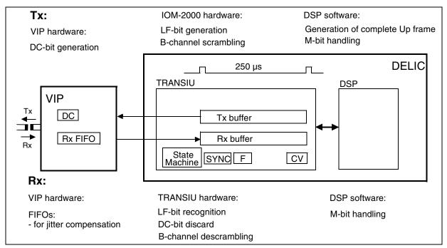
Figure 24 Handling of U<sub>PN</sub> Frame (one Channel)
