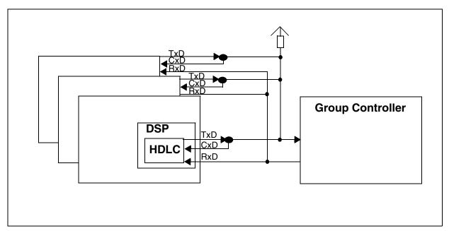
Figure 48 Point-to-Multi Point Bus Structure
