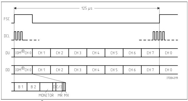
Figure 19 IOM®-2 Interface in Digital Line Card Mode
