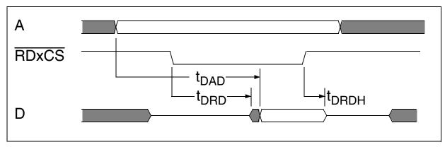
Figure 66 Read Cycle Intel/Infineon Demultiplexed Mode
