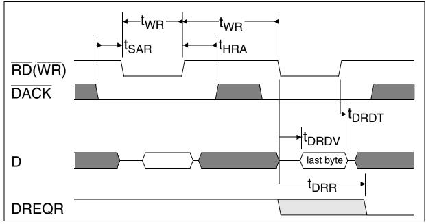
Figure 62 DMA Read-Transaction Timing in Intel/Infineon Mode
