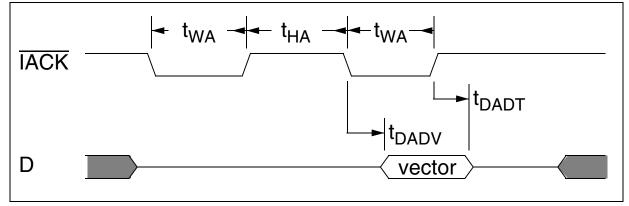
Figure 70 Interrupt Acknowledge Cycle Timing in Intel/Infineon Mode
