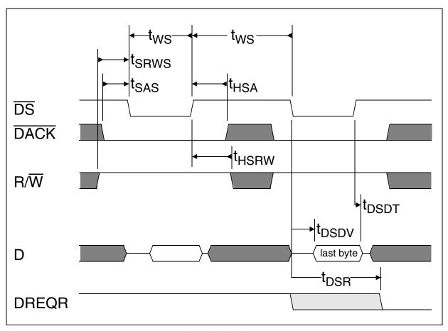
Figure 60 DMA Read-Transaction Timing in Motorola Mode
