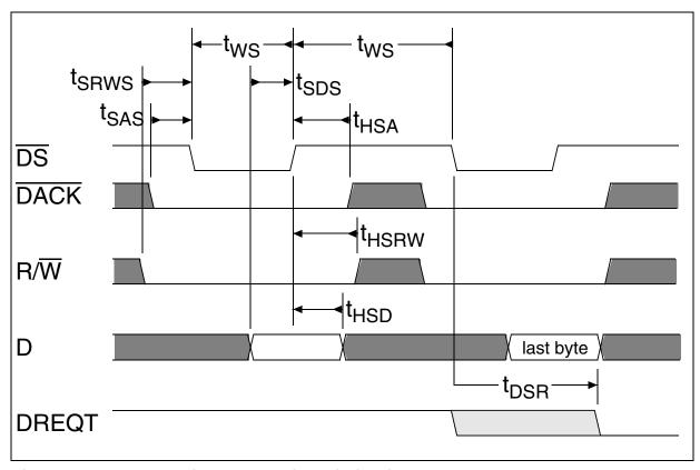
Figure 59 DMA Write-Transaction Timing in Motorola Mode
