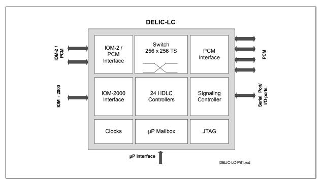
Figure 1 Block Diagram of the DELIC-LC
