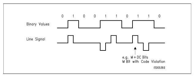
Figure 23 AMI Coding on the Up Interface
