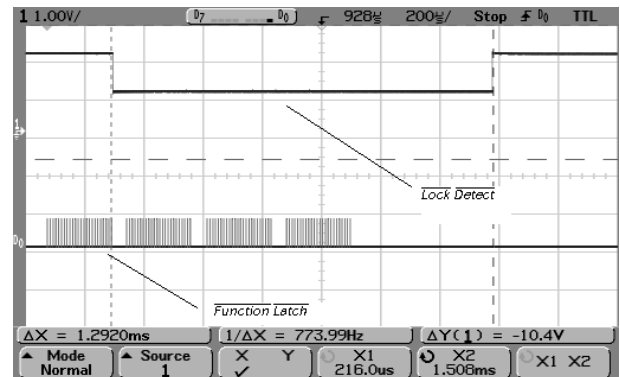
Start-up time for ADF7010 from Function Latch being programmed to Lock Detect going high, Vdd = 3V
