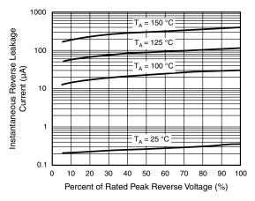
Figure 6. Typical Reverse Leakage Characteristics Per Diode
