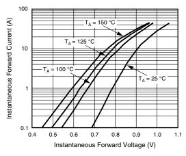
Figure 5. Typical Instantaneous Forward Characteristics Per Diode
