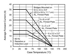
Figure 1. Maximum Output Rectified Current
