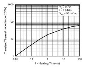
Figure 8. Typical Transient Thermal Impedance Per Diode
