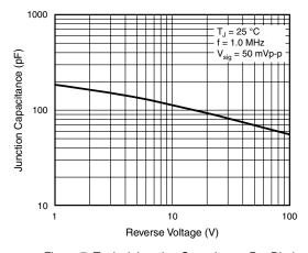
Figure 7. Typical Junction Capacitance Per Diode
