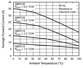
Figure 2. Maximum Output Rectified Current
