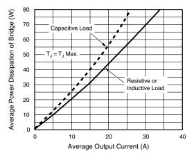
Figure 3. Maximum Power Dissipation
