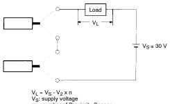
n: number of Proximity Sensor V<sub>2</sub>: residual voltage
