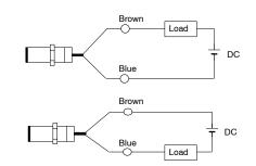
Note: It is possible to connect the load in two ways as shown in the above diagrams.
