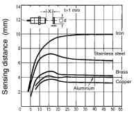
Side length of sensing object (mm)
