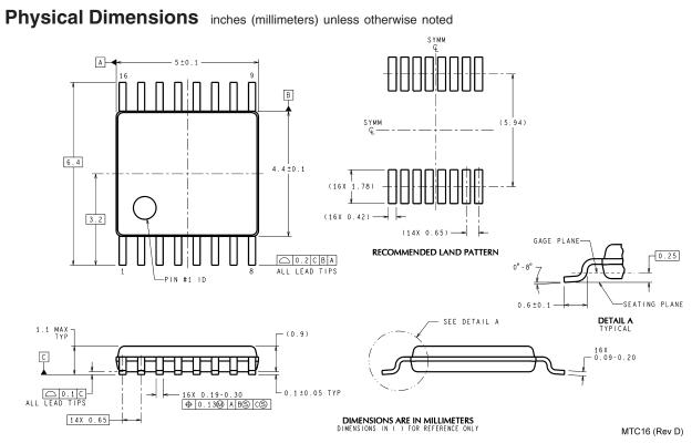
Dimensions are in millimeters.
