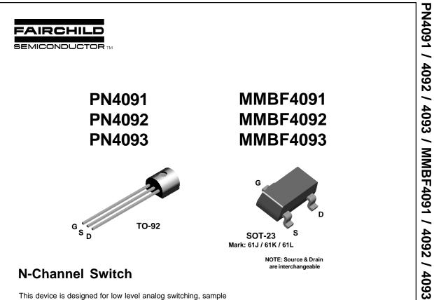
This device is designed for low level analog switching, sample and hold circuits and chopper stabalized amplifiers. Sourced from Process 51. See J111 for characteristics.
