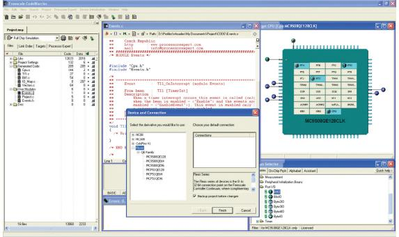
appropriate support files (header files, libraries and linker files). For projects switching between 8-bit and 32-bit Flexis™ series microcontrollers this is the extent of the porting effort.
