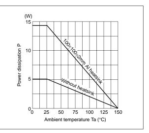
When selecting a heatsink for SLA5017, be sure to check the product temperature when in use in an actual application. The calculated loss is an approximate value and therefore con-
