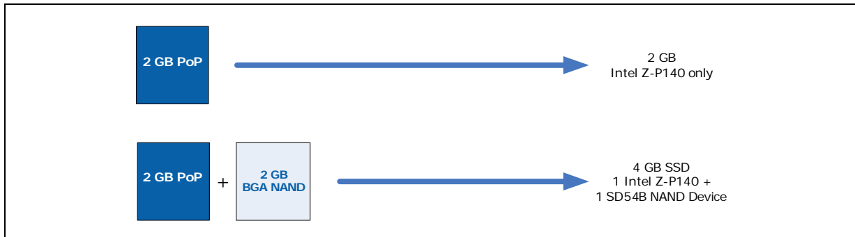
Figure 3. 2 GB Configuration Using Intel SD54B NAND Flash Memory
