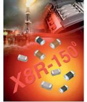
AVX have developed a range of multilayer ceramic capacitors designed for use in applications up to  $150^{\circ}$ C. These capacitors are manufactured with an X8R dielectric material which has a capacitance variation of  $\pm 15\%$  between -55°C and  $\pm 150^{\circ}$ C.
