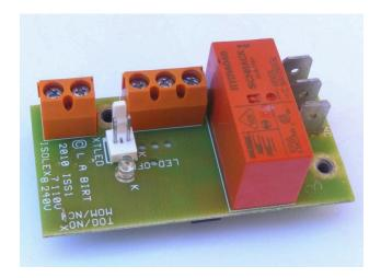
At last, a 21<sup>st</sup> century, low cost alternative **to air switch systems and tubing**. These AC powered, miniature (60 X 30 mm) units utilise advanced ferro-magnetic technology to provide **full galvanic isolation to connected electrical switches**. The novel, low impedance technique, passes near zero current through the connected switch creating a safe, earthed **'electric free'** circuit.
