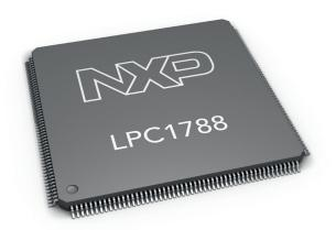
120 MHz, 32-bit MCUs with Cortex-M3™ core LPC177x / LPC178x series
