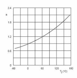
$a = \frac{R_{DSon}}{R_{DSon(25^{\circ}C)}}$
