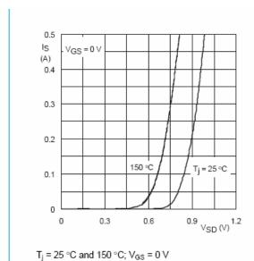
Fig 12. Source (diode forward) current as a function of source-drain (diode forward) voltage; typical
