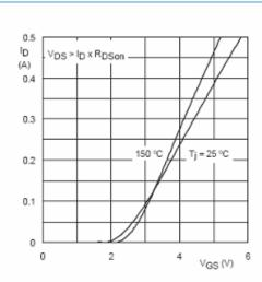
$T_j = 25$  °C and 150 °C;  $V_{DS} > I_D \times R_{DSon}$
