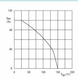
$$I_{der} = \frac{I_D}{I_{D(25^{\circ}C)}} \times 100\%$$
