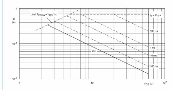
$T_{sp}$  = 25 °C;  $I_{DM}$  is single pulse;  $V_{GS}$  = 10 V
