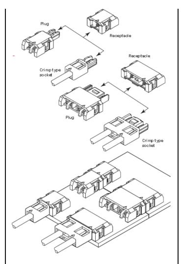
Designed for LED light bar applications, the low profile of the connector does not interfere with the *luminescence* angle of LED dies. The LEB Series provides both board-to-board and wire-to-board capabilities. The board-to-board plug and receptacle connectors allows continuous connection of LED light bars
