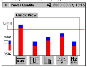
This quick view summarises measurements to give a pass / fail indication. The 95% value indicates measurements within 95% of the allowable limits
