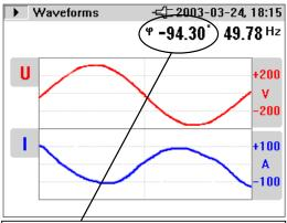
Phase angle between voltage and current is displayed in degrees.
