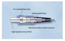
cian influence to a minimum. On site, the stripped and cleaved field fibres are inserted into the UniCam connectors and retained. A mechanical splice inside the connector establishes the low-loss connection between the field fibre and the preinstalled fibre inside the connector.
