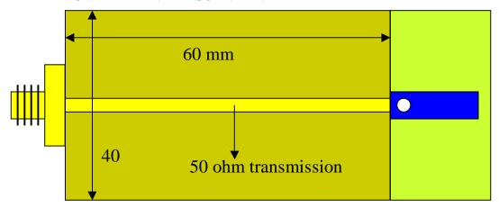
FR-4 PCB thickness = 0.8 mmThe length of transmission line = 60 mm ( depends on PCB thickness)
