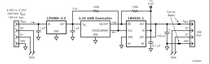
FIGURE 3. Single-Port USB Self-Powered Hub
