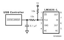
FIGURE 1. Transient Fitter
