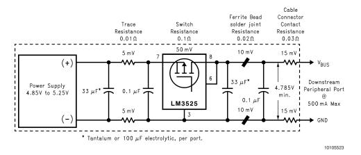
FIGURE 2. Self-Powered Hub Per-Port Voltage Drop
