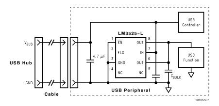
FIGURE 5. Inrush Current-limit Application
