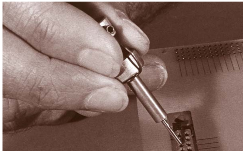
INSERT EXTRACTION TOOL WITH PLUNGER RETRACTED
