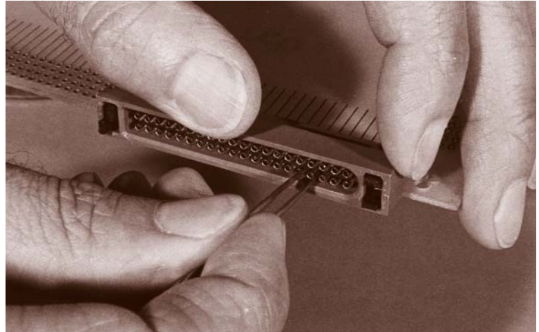
REMOVE DAMAGED CONTACT
