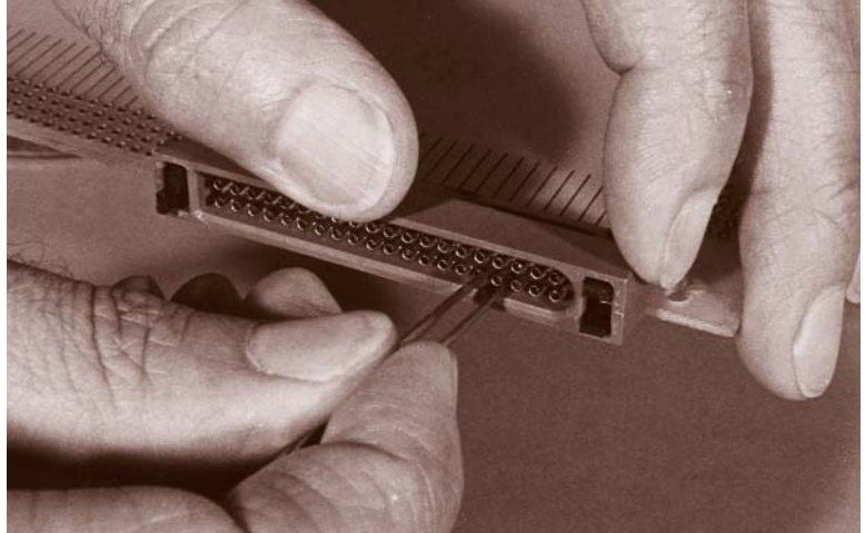
REMOVE DAMAGED CONTACT
