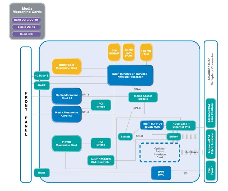
Figure 1: Intel® IXMB2805 or Intel® IXMB2855 Single Network Processor Base Card Functional Block Diagram
