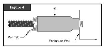
**5.** Position Cold Shrink Corrosion Protection Assembly (*Figure 4*) over bulkhead termination connector. Install by unwinding loose core pull tab in a counter-clockwise direction around cable. Rubber sleeve should make contact with enclosure wall during installation.
