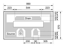
**Remark** Chip thickness:  $100 \mu m$  G : Gate
