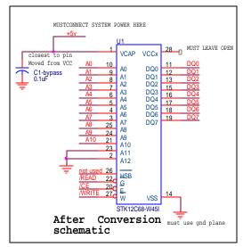
On the next page, pin by pin comparisons of the two show all pins are the same except for the bypass capacitor moving to pin 1 and connected to system power, +5v. Pin 28 must now be unpowered and open.
