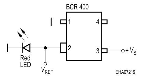
Precision timer with BCR400 providing constant charge current
