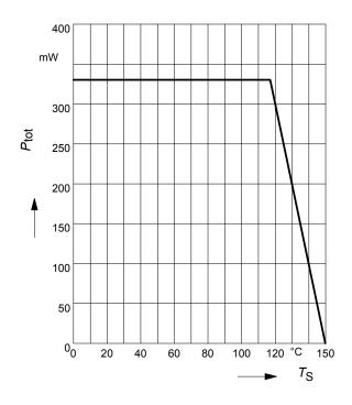
Note that up to  $T_{S}$ =115°C it is not possible to exceed  $P_{tot}$ respecting the maximum ratings of  $V_{S}$  and  $I_{Contr.}$ The collector or drain current (respectively) of the stabilized RF transistor does not affect BCR 400 directly, as it provides just the base current.
