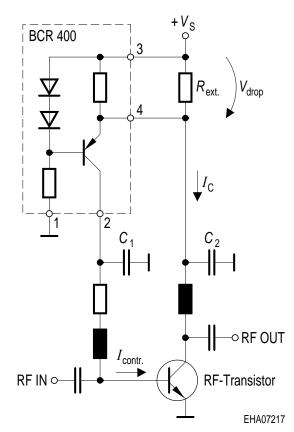
Be aware that BCR400 stabilized bias current of transistors in an active control loop
