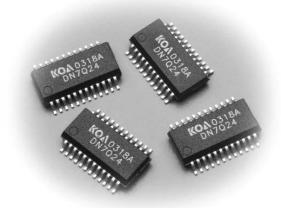
This diode network is designed to provide eighteen channels for active termination of high-speed data signals to eliminate signal undershoot and overshoot. The network has the added benefit of acting to suppress any ESD voltage events by shunting the energy to ground assuring maximum reliability of electronic systems in the field. Trigger levels are defined by the positive and negative bias levels set by the user.
