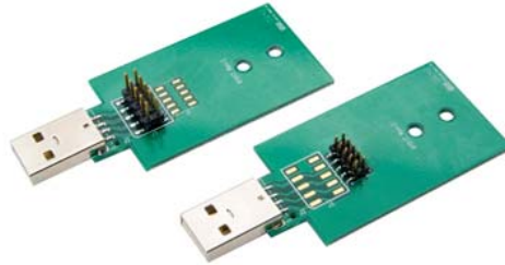
Figure 5: USB Flash Disk Module 2x5 Adapters
