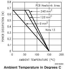
Note: ( $P_{DMAX} = 670$ mW for 5V, 8 $\Omega$ )
