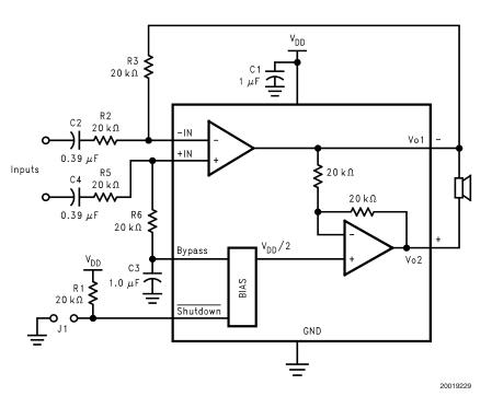
FIGURE 3. DIFFERENTIAL AMPLIFIER CONFIGURATION FOR LM4890
