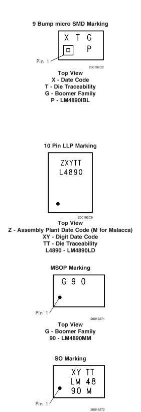
Top View XY - Date Code TT - Die Traceability Bottom 2 lines - Part Number
