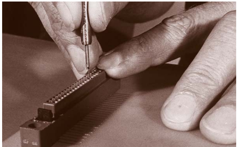
SEAT CONTACT WITH INSERTION TOOL
