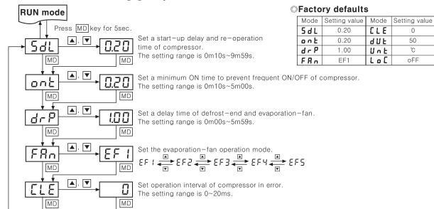
Set the ON operation ratio(%) of compressor within operation interval in error. The setting range is 0~100%.
