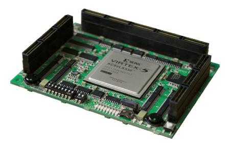
The Logic Tile for the Xilinx XC5VLX330 FPGA is implemented in a 65-nanometer process with wider Look-Up-Tables inputs (6-input LUTs), which reduce critical path delays, facilitating timing closure for ASIC prototyping. It has the same I/O interconnect as the Logic Tiles for the Xilinx Virtex-4 FPGA with a maximum clock frequency and capacity increase, making system partitioning easier. The Logic Tile for the Xilinx Virtex-5 FPGA also features an on-board 32MB ZBT SRAM.
