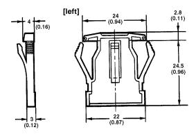
Note: End caps are attached to each end of the switch assembly and used to secure the switch assembly to a mounting panel.
