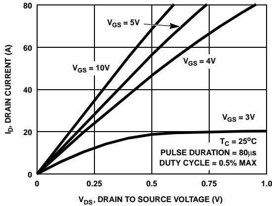
**Figure 8. Saturation Characteristics**
