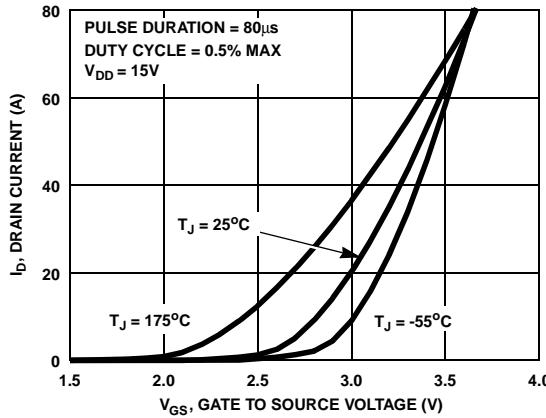
**Figure 7. Transfer Characteristics**
