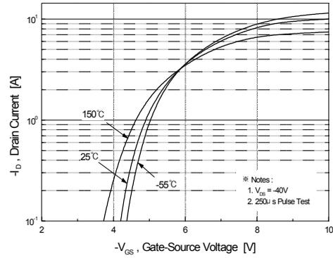
Figure 2. Transfer Characteristics
