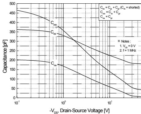
Figure 5. Capacitance Characteristics
