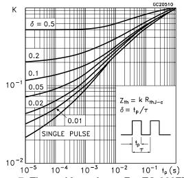
Figure 7: Thermal Impedance For TO-220FP
