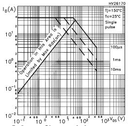
**Figure 5: Output Characteristics**
