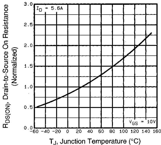
**Fig 4.** Normalized On-Resistance
