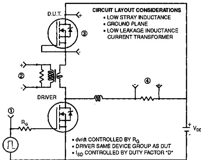
Fig 14. Peak Diode Recovery  $dv/dt$  Test Circuit
