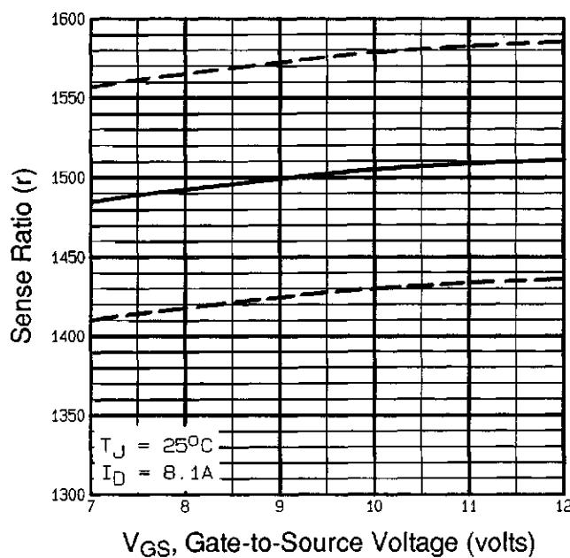
**Fig 17.** Typical HEXSense Ratio Vs. Gate Voltage
