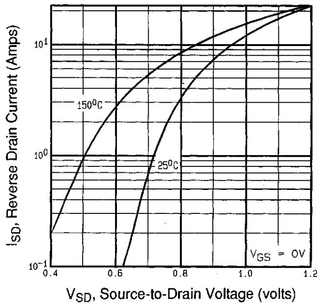
**Fig 7.** Typical Source-Drain Diode
