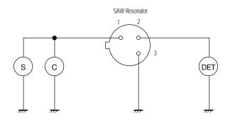
**Standard measuring voltage:** –6 dBm between pins 1 and 2 (0.112 Vrms)
