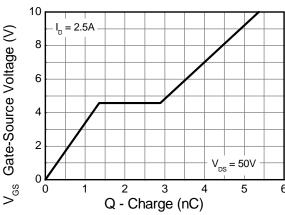
**Gate-Source Voltage v Gate Charge**
