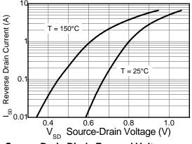
Source-Drain Diode Forward Voltage
