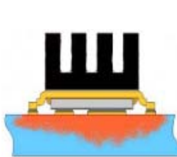
③ Mounted to a PCB with small clip heatsink (still air)
