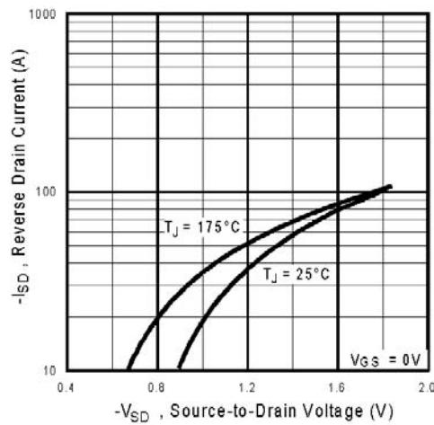
**Fig 7.** Typical Source-Drain Diode
