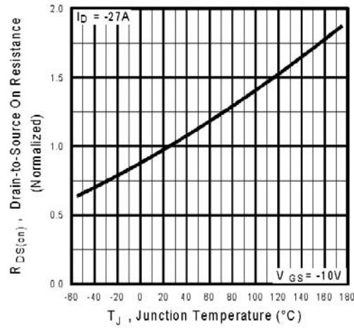
**Fig 4.** Normalized On-Resistance
