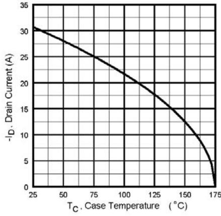
**Fig 9.** Maximum Drain Current Vs.
