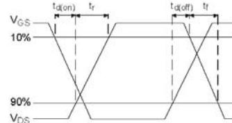
**Fig 10b.** Switching Time Waveforms
