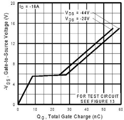
**Fig 6.** Typical Gate Charge Vs.
