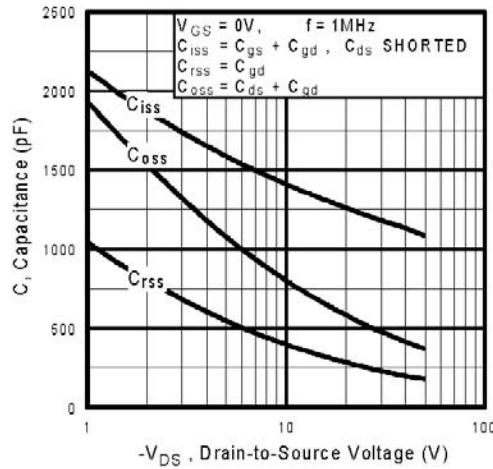
**Fig 5.** Typical Capacitance Vs.
